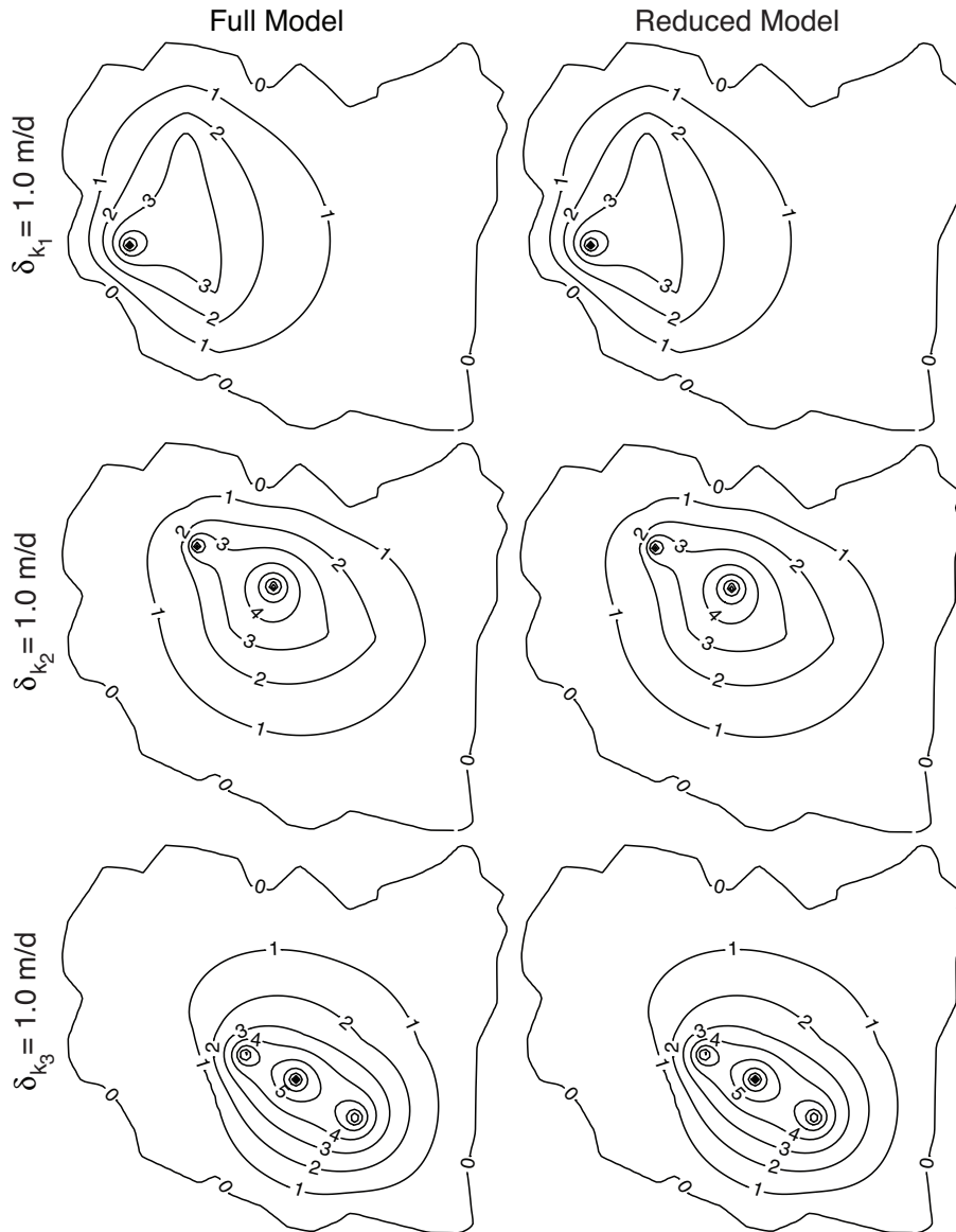
Figure 3.6: Changes in drawdown (m) given a unit change in hydraulic conductivity (1.0 m/d) for both the linearized full and reduced models.
