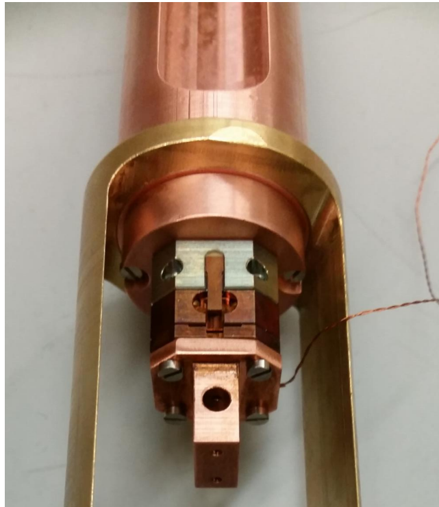
Figure 4.9: Completed Design: Attocube stage with mounting plate and sample mount. This setup is now in the dilution fridge experimental setup.
