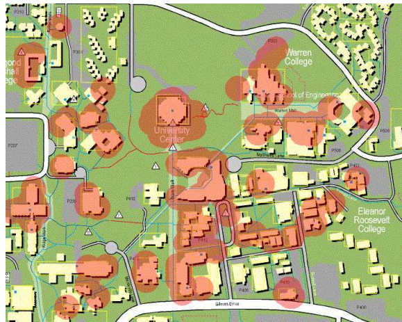
Figure 1: A map of wireless coverage over a large University campus. The entire coverage area is serviced by over 250 distinct access points
