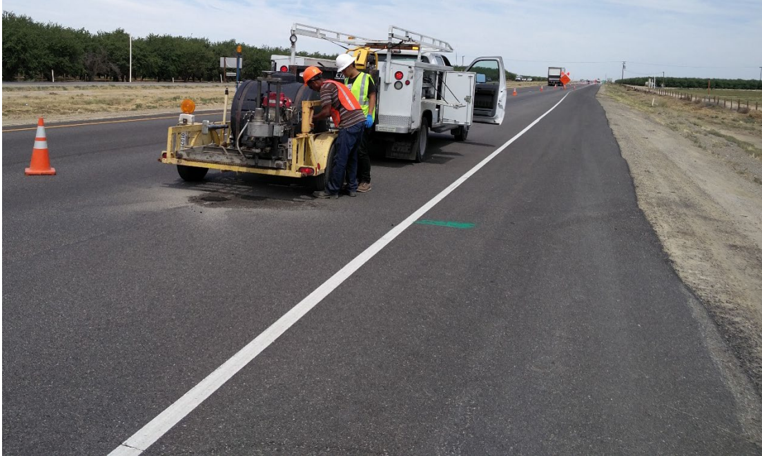
Figure A.40: PH19 On-site location photograph during coring pavement sample under Caltrans closure.
