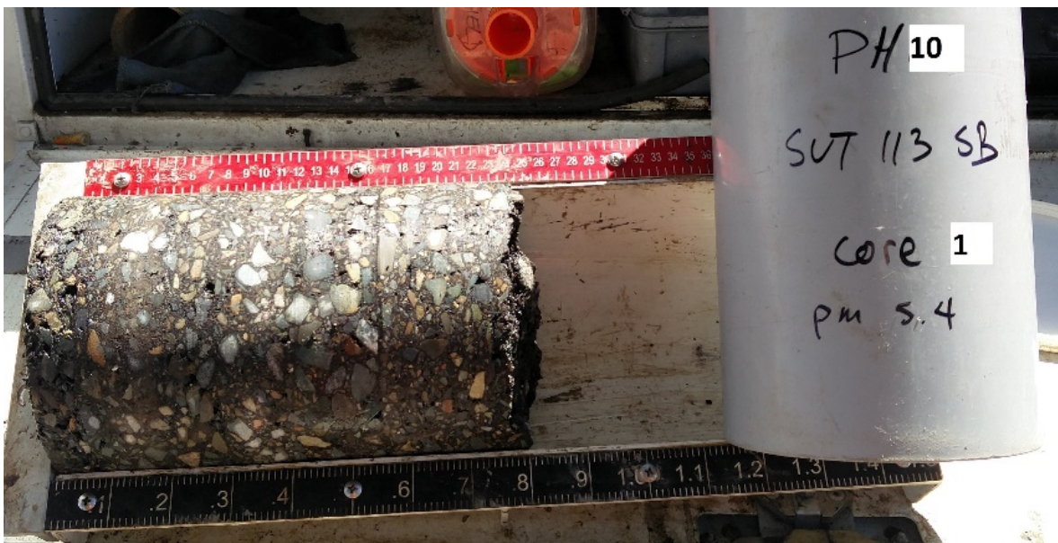
Figure B.13: Pavement core sample for PH10.
