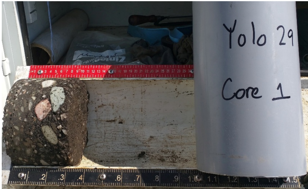
Figure B.8: Pavement core sample for PH08.
