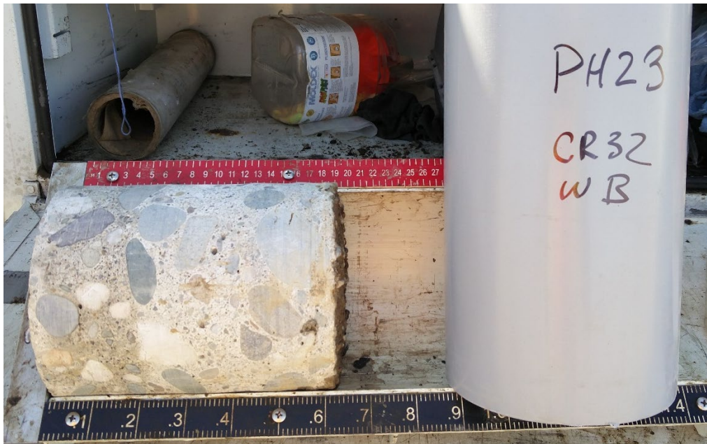
Figure B.38: Pavement core sample for PH23.
