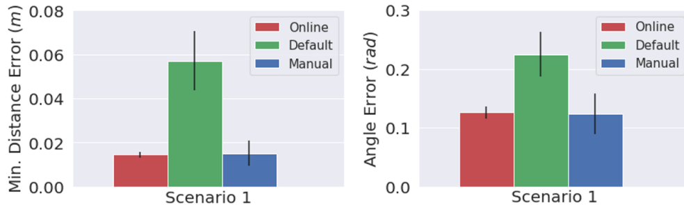
Figure 4.11: Effects of varying linear acceleration bound for real-world experiments. Best bound found is 0.3 m/s^2 .
