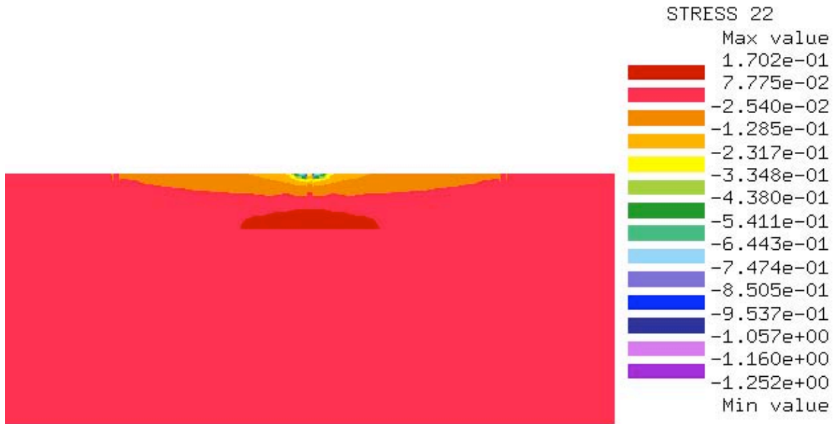
Figure 6.8: Normal transverse stress component; transverse plane through the plugs' centers.
