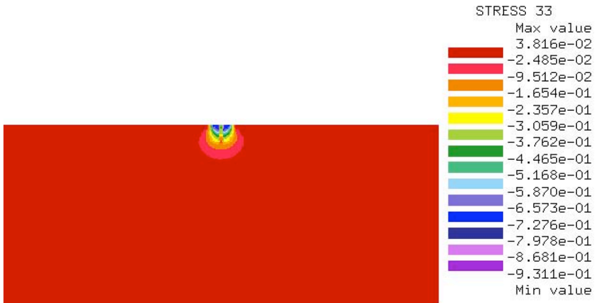
Figure 6.9: Normal vertical stress component; transverse plane through the plugs' centers.
