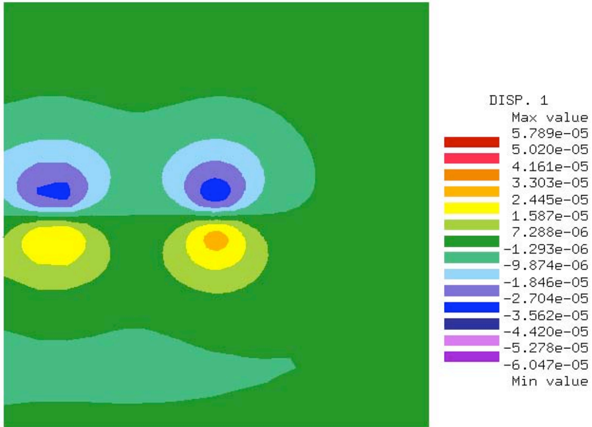
Figure 6.30: Longitudinal disp. contours; AC surface; traffic loading (S25); Palmdale; S1.
