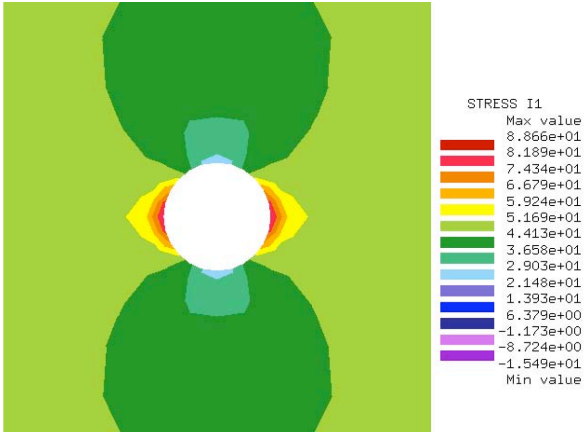
Figure 6.20: I_1 contours on the surface of the AC layer; thermal loading; Fairbanks; S1.
