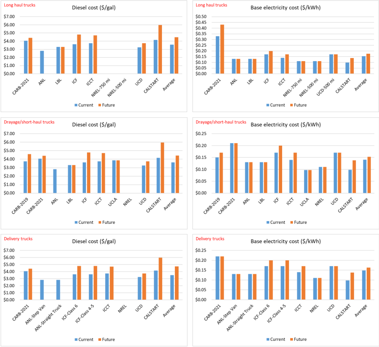
Figure 19. Fuel/energy cost comparison across studies and truck types (diesel in $/gal and electricity in $/kWh)
