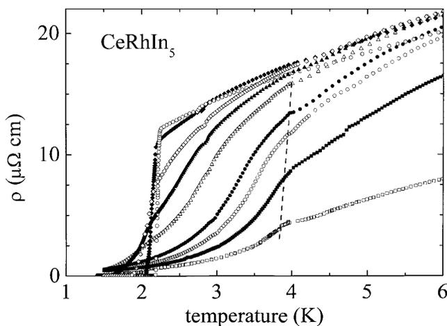
FIG. 3. Low-temperature response of CeRhIn<sub>5</sub> to applied pressures. With increasing resistivity at 2.3 K, the curves correspond to applied pressures of 0.001, 7.9, 9.9, 12.2, 14.5, 16.3, 17.2, 18.5, and 21.0 kbar. The diagonal dashed line is a guide to the eye.
