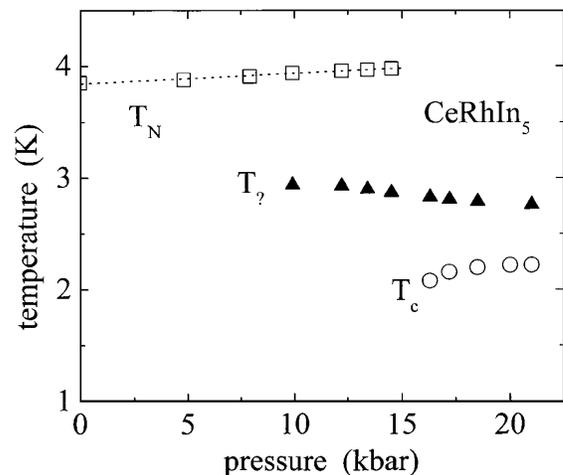
FIG. 4. Temperature-pressure phase diagram for CeRhIn<sub>5</sub> constructed from data shown in Fig. 3. Squares and circles give the pressure dependence of the Néel and onset superconducting transition temperatures, respectively. Triangles correspond to resistance features of unknown origin; see text. The dashed line has a slope of 9 mK/kbar.
