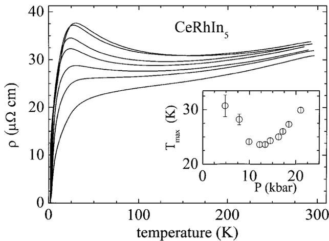
FIG. 2. Temperature dependence of the electrical resistivity of CeRhIn<sub>5</sub> at representative applied pressures. Data shown correspond to pressures of 0.001, 4.8, 7.9, 12.2, 14.5, 18.5, and 21.0 kbar and are associated, respectively, with curves of increasing resistivity at 50 K. The inset is a plot of the pressure dependence of the temperature  $T_{\max}$  where the resistivity is a maximum.
