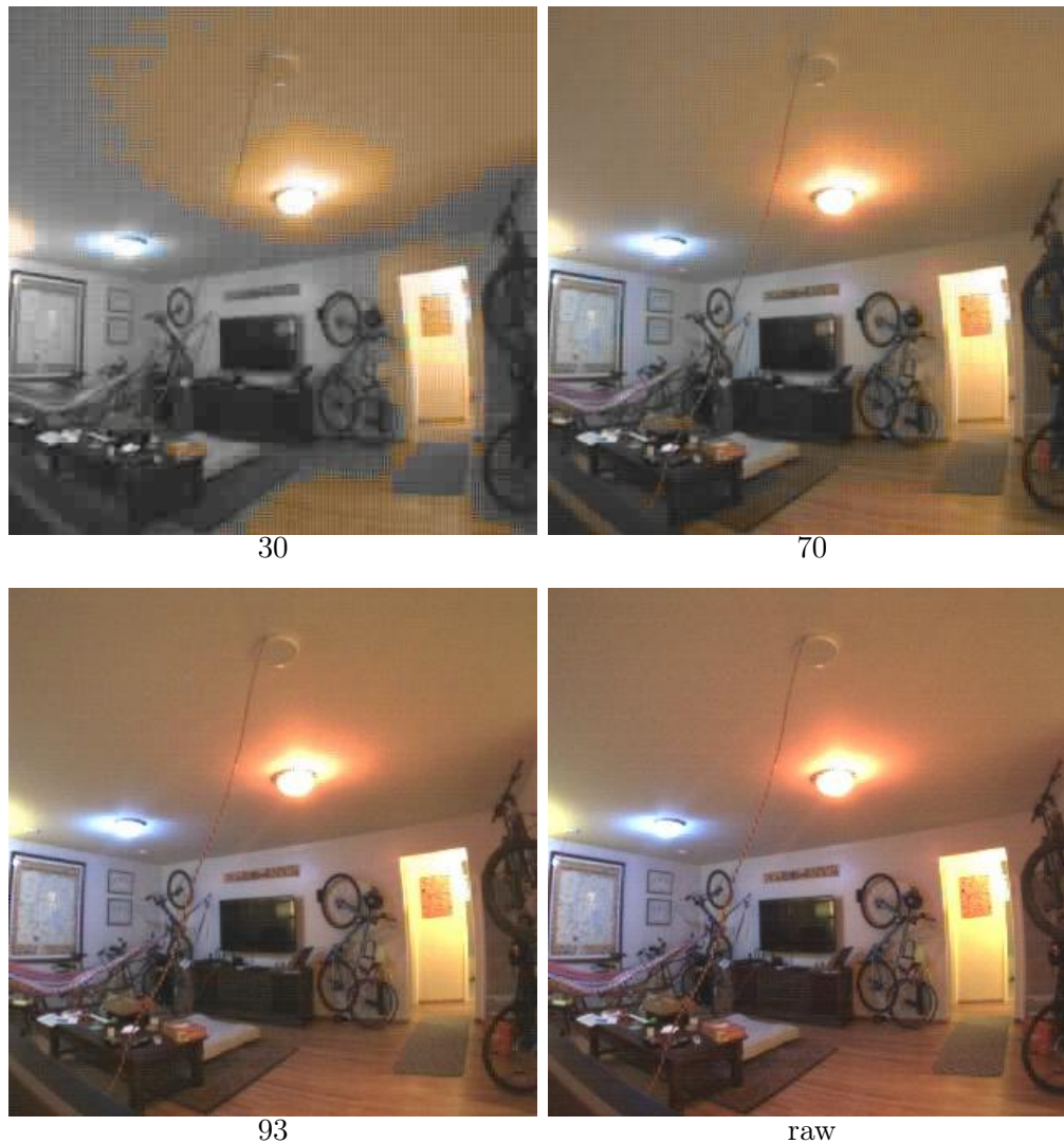
Figure 6.13: An image compressed with different quality factors. In this scene, we set smart lights to bright, intense colors to determine the effects of compression on color representation. Compression is performed on the mosaiced version of the image, which after transmission is demosaiced into the color representations displayed. Due to this, an image compressed with a low quality factor loses significant color information compared to the raw image. Luckily, high quality factors produce a near-indistinguishable representation of the raw image. We explore a more quantitative view of image similarity in Figure 6.14.
