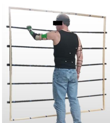
Figure 2. Experimental setup with a transradial limb-different participant. Participants were requested to sequentially power-grasp 7 x 7 equally spaced targets on the beams of the grid. The image shows the target grid in horizontal configuration. The experiment was repeated with the grid rotated 90 degrees into a vertical configuration. This rotation alters the target grasp orientation.
