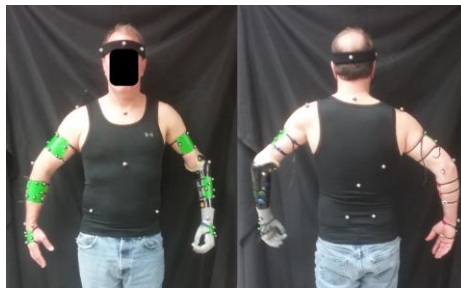
Figure 6: Motion capture marker configuration on an amputee participant, using a combination of marker clusters (attached to flexible sheet plastic) and individual markers.
