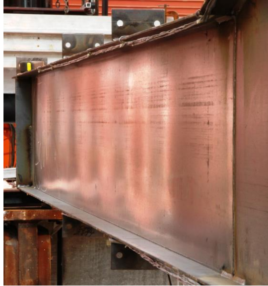
Figure 6.2 Web Geometric Imperfection (Smith et al. 2013)
