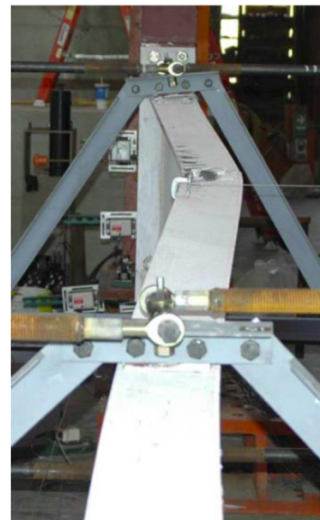
Figure 1.2 Global and Local Buckling Interaction with LTB (Smith et al. 2013)
