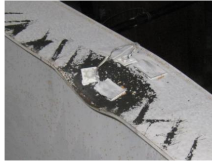
(b) Inner Flange FLB at Mid-Length of CS
