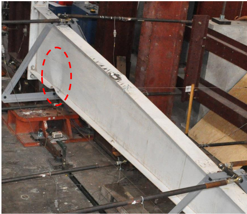
Figure 5.15 CS1 Outer Flange FLB and WLB (-4.8 in., 1 st Cycle)
