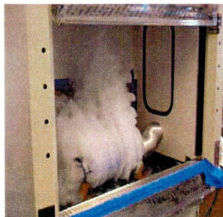
Figure 11. Berkeley Hood, showing full containment.
