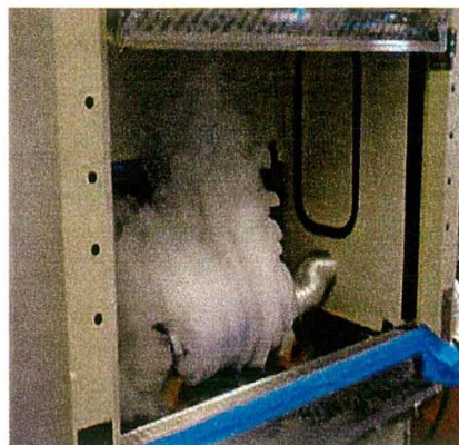
Figure ES-4. High-performance Berkeley Hood, showing full pollutant containment.
