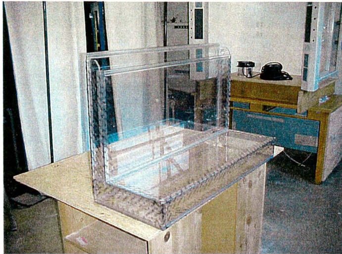
Figure 5. Clear plastic plenum to facilitate visual tests
