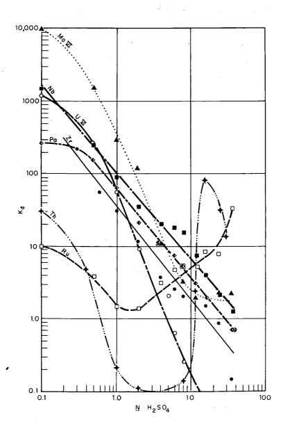
Figure 7 Equilibrium adsorption of thorium and several other elements by Dowex-2 from sulfuric acid solution. Data from Bunney, Ballou, Pascual and Foti $^{57}$ .
