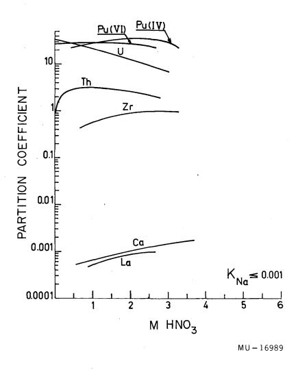
Figure 2 Solvent extraction data for methyl isobutyl ketone. The distribution ratios of U, Pu, Th, Zr, La and Ca as functions of the equilibrium concentration of  $\mathrm{HNO}_3$  in the aqueous phase. Concentration of  $\mathrm{Ca(NO}_3)_2$  is 3.5 to 4.0 Molar. Data by Rydberg and Bernström.  $^{27}$
