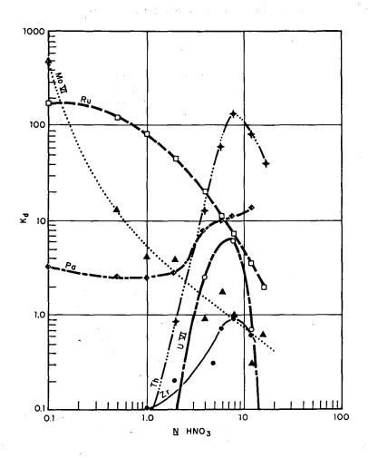
Figure 6 Equilibrium adsorption of thorium and several other elements by Dowex-2, 8 percent DVB, 200-400 mesh from nitric acid. Data from Bunney, Ballou, Pascual and Foti<sup>57</sup>.
