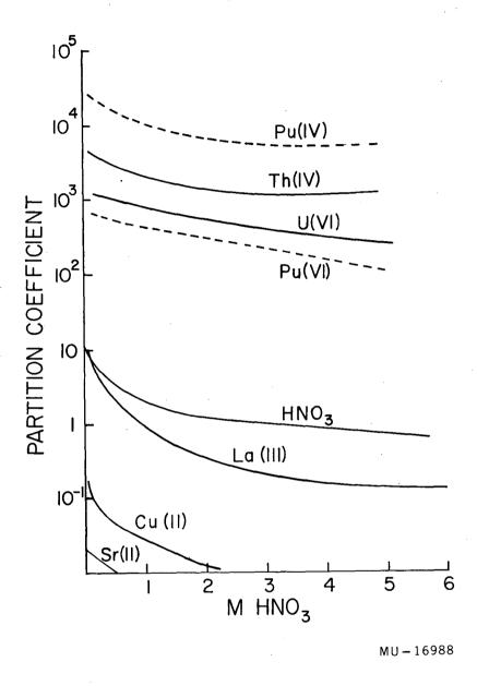
Figure 5 The partition coefficients (org/aq) of Th(IV) and of several representative contaminating ions into undiluted TBP as a function of  $\text{HNO}_3$  in the aqueous phase. The aqueous phase concentration of  $\text{Ca(NO}_3)_2$  is fixed at 3 Molar. The curves for Pu(VI) and Pu(IV) have been extrapolated assuming Pu(VI) parallels U(VI) and Pu(IV) parallels Th(IV). From Bernström and Rydberg 141.
