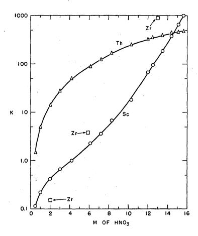
Figure 4 Variation of distribution ratios (TBP/aqueous) of scandium, thorium and zirconium with aqueous HNO concentration for extraction into pure undiluted TBP. Peppard, Mason and Maier 42.
