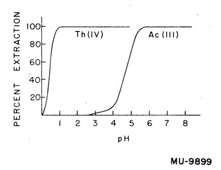
Figure 1 Extraction of trace amounts of actinium and thorium from a dilute nitric acid solution by an equal volume of an 0.25  $\underline{\text{M}}$  solution of TTA in benzene as a function of pH.
