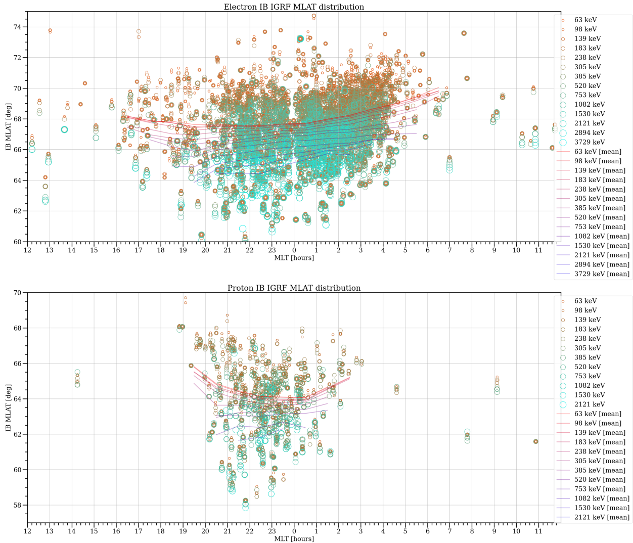
Figure 5.2: MLT scatter plot of ELFIN electron IB events (top) and proton IB events (bottom) in each energy channel. The radius of the circular markers is scaled linearly with the energy channel, allowing for identification of energy-latitude dispersion patterns within the same event. Note: the electron IB scale is at higher latitude than for protons.
