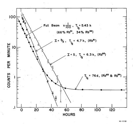
Fig. 11. The decay curves of the Rb 81 and Rb 82 resonances compared to the normal beam sample.
