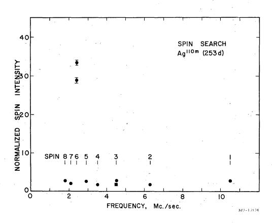
Fig. 8. Spin search for Ag 110m. The ordinate is the counting rate, the abscissa is exposure frequency.
