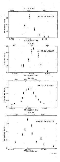
Fig. 17. Tl<sup>204</sup> resonances as a function of increasing magnetic field. The scale of equivalent hyperfine separations is at the top of each graph.
