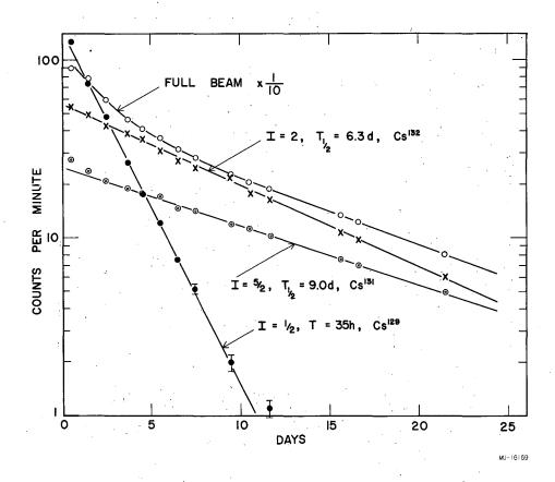
Fig. 12. The decay curves of the Cs 129, Cs 131, and Cs 132 resonances compared to the normal beam sample.
