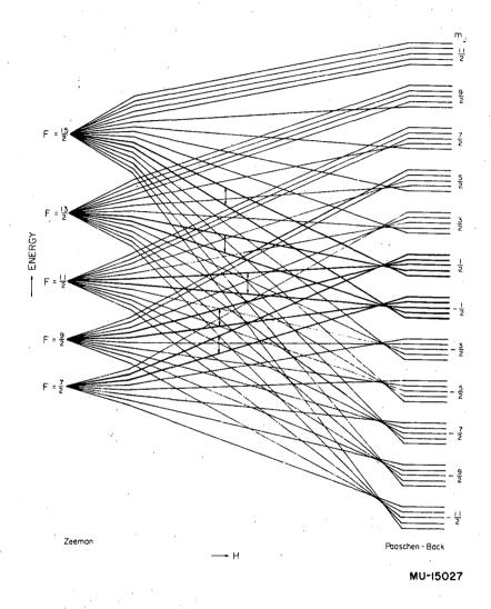
Fig. 19. Breit-Rabi diagram for J = 11/2, I = 2 as for neptunium-238.
