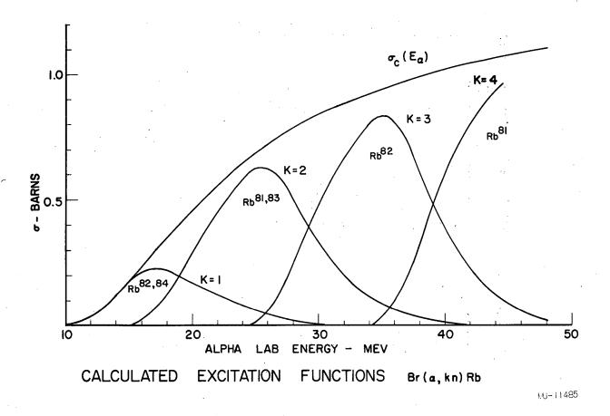
Fig. 10. Production curve for rubidium isotopes as a function of the alpha-particle energy.
