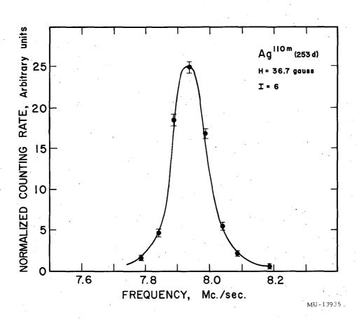
Fig. 9. Resonance line shape of Ag 110m.
