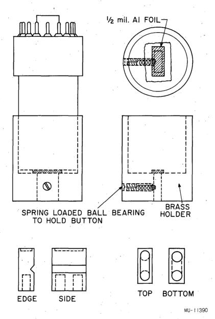
Fig. 7. X-ray counters and collecting button.
