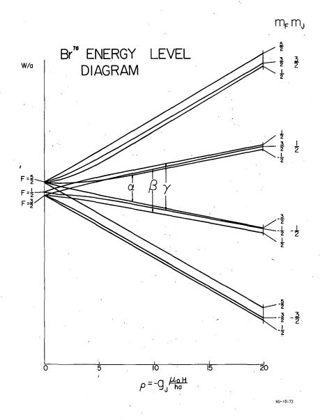
Fig. 18. Breit-Rabi diagram for J = 3/2, I = 1, inverted as for Br 76.
