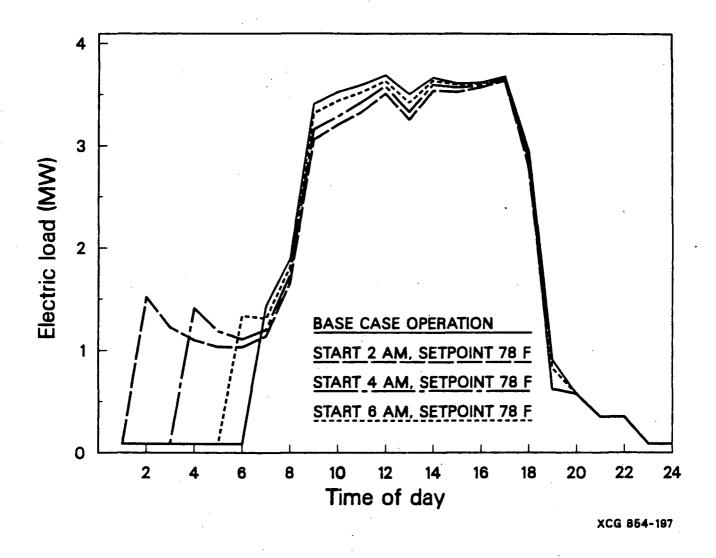
Figure 4. Electric load profiles for load-shifting, pre-cooling strategies.
