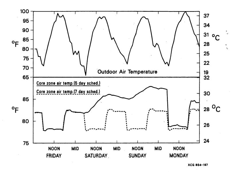
Figure 1. Outdoor dry-bulb air temperature and indoor core air temperatures for 5- and 7-day schedules of building operation.
