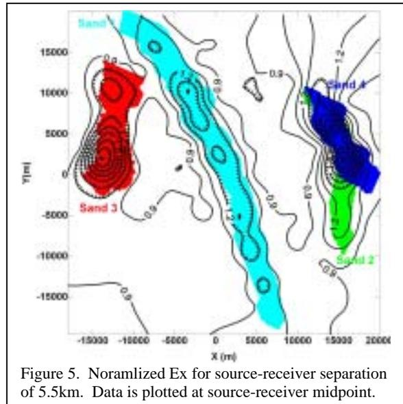
Figure 5. Normalized  $E_x$  for source-receiver separation of 5.5km. Data is plotted at source-receiver midpoint.
