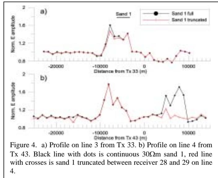
Figure 4. a) Profile on line 3 from Tx 33. b) Profile on line 4 from Tx 43. Black line with dots is continuous 30 $\Omega\text{m}$  sand 1, red line with crosses is sand 1 truncated between receiver 28 and 29 on line 4.
