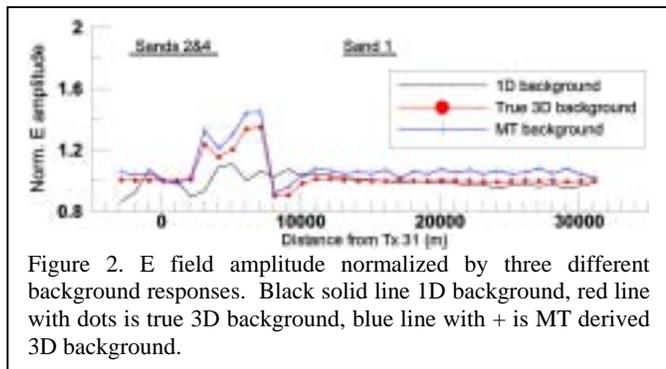
Figure 2. E field amplitude normalized by three different background responses. Black solid line 1D background, red line with dots is true 3D background, blue line with + is MT derived 3D background.
