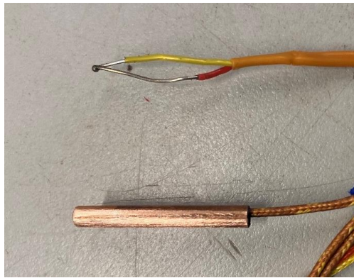
Figure 5-23: a) Cross sectional diagram of the brake shoe backing plate and lining material with installed thermocouples probes with a gap of 1.9 mm and 5.2 mm from the surface. b) Image of the probe tips, one exposed (top) and a second enclosed (bottom), used during bench top tests.
