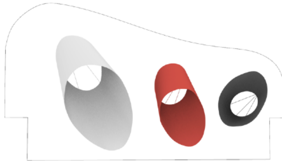
Figure 5.3 A view from the bottom of the “light cannons” with the ceiling contour. The white “light cannon” on the east grows towards the northeast. The red “light cannon” in the middle extrudes to the north. And the black one on the west points its tip to the northwest. (Digital reconstruction by author in March 2022).
