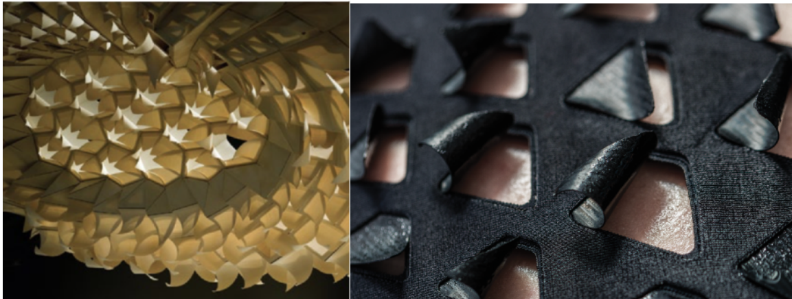
Figure 6.8 Humidity responsive. Left: HygroScope: Meteorosensitive Morphology , Achim Menges and Steffen Reichert, 2012. (Source: http://www.achimmenges.net/?p=5083 ). Right: Macroscopic view of the bio- hybrid film that reacts to sweaty skin. (Source: https://tangible.media.mit.edu/project/biologic/ ).
