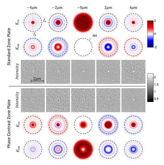
Fig. 2. Sample measurements taken using the standard zone plate (top) and phase contrast zone plate (bottom). The defocus distance is indicated at the top, along with the real and imaginary transfer functions in frequency space for each image, with the NA marked by a dashed circle. The illumination is a disk source with  $\sigma = 0.25$ .
