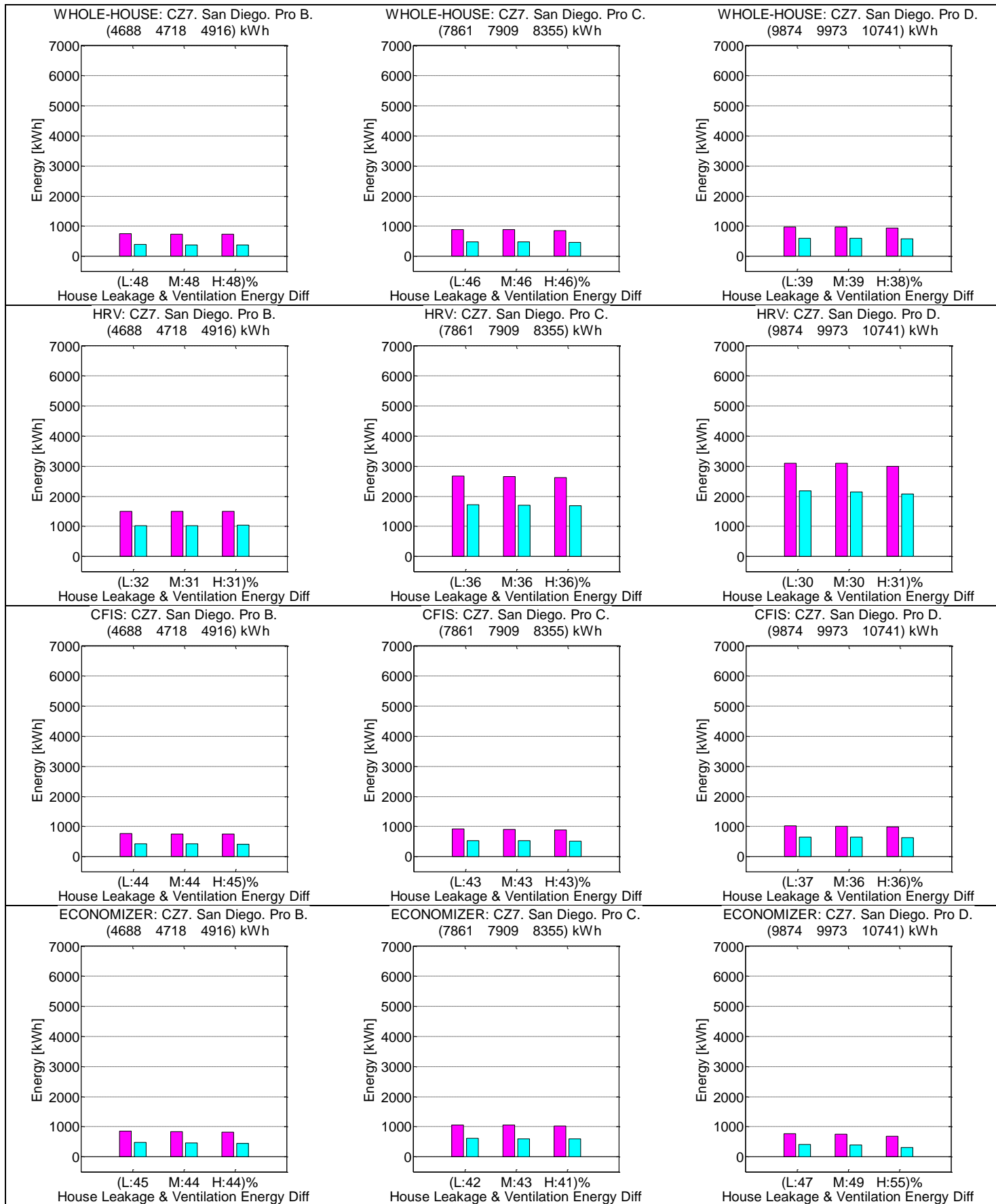
Figure 35: Ventilation-related energy penalty with and without RIVEC for climate zone 7, San Diego
