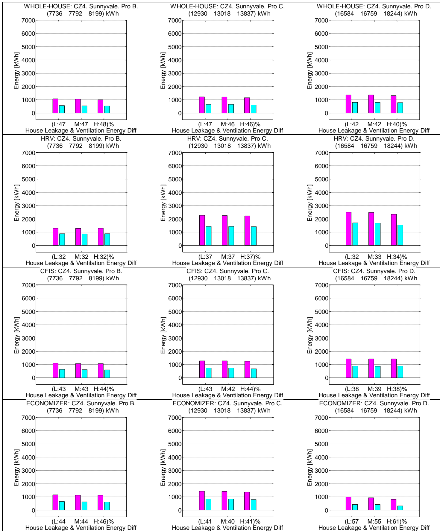
Figure 32: Ventilation-related energy penalty with and without RIVEC for climate zone 4, Sunnyvale
