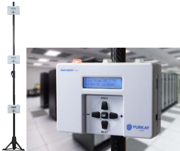
Figure 3.2.1: AUDIT-BUDDY Tool: Three Temperature/Humidity (TH1) Units Mounted on a Carbon Fiber Rod
