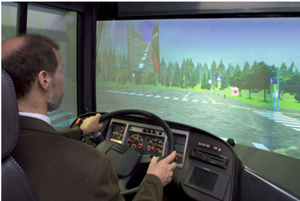
Figure 5. Truck eco-driving training in driving simulator environment [photo credit: https://www.iru.org/en_policy_co2_response_ecodriving ]
