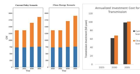
Figure 3. Interprovincial and interregional transmission capacity (left panel) and annualized costs for new transmission (right panel)
