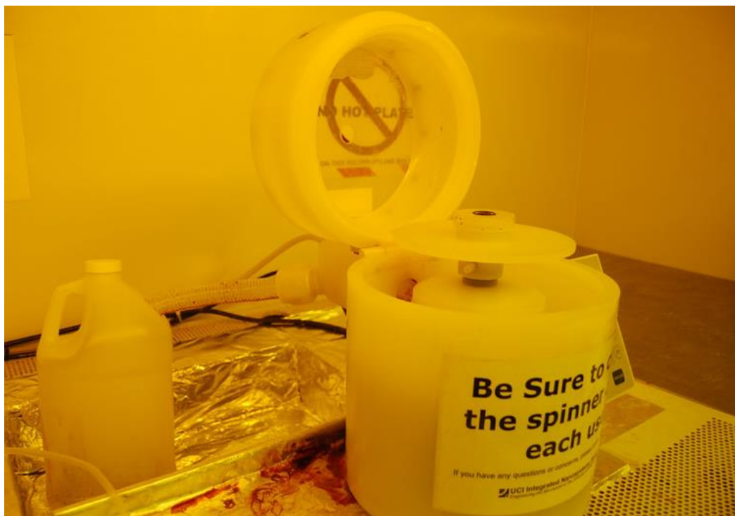
Figure 10: Programmable Laurell photoresist spinner Courtesy: UCI Bio-Organic Nanofabrication facility
