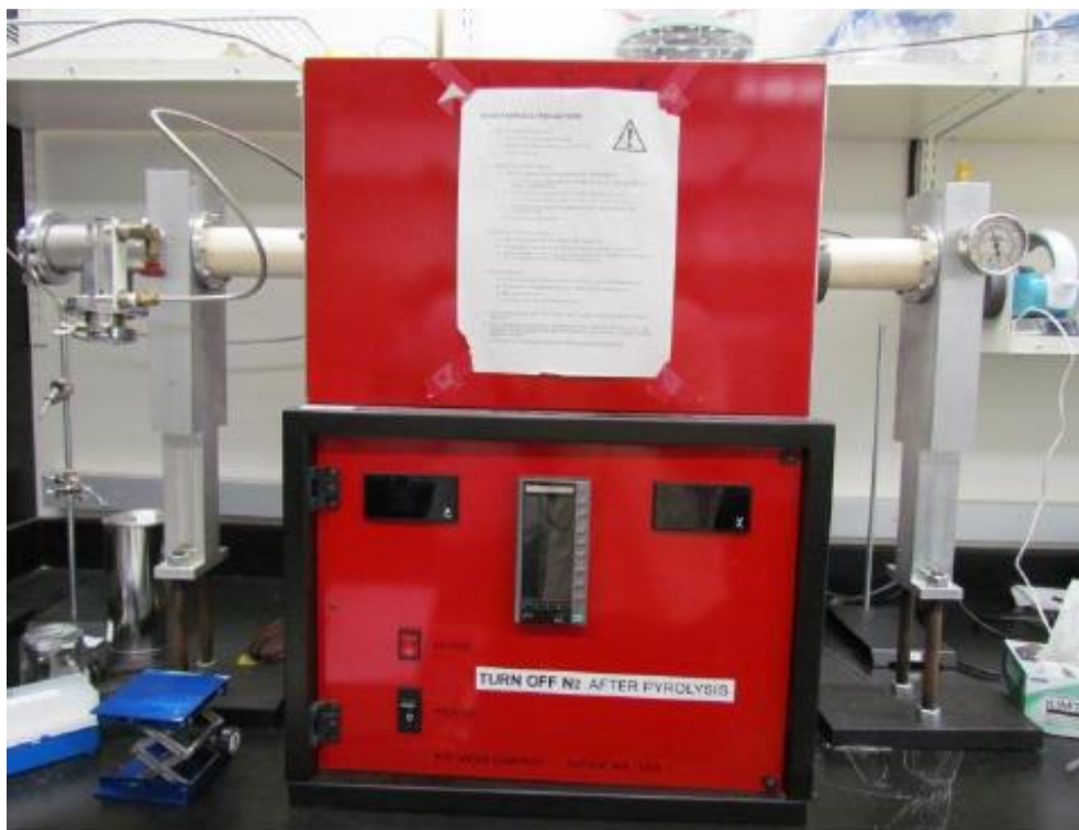
Figure 13: RD Webb Mini Furnace with alumina tube for pyrolysis
