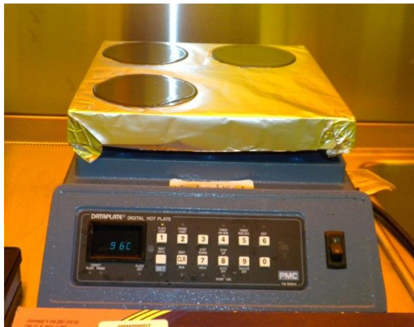
Figure 11: A programmable hot plate for soft bake and postbake.
