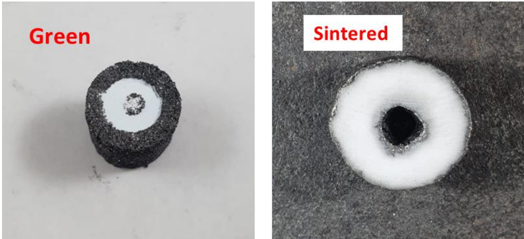
Figure 7.2.1.1: Initial experimental results with one channel. The printed graphite scaffold with HAP powder inside (left) and the final sample after SPS (right).
