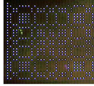
Figure 2. A magnified photograph of the 58 x 58 NTHT used in the coded aperture imaging of fluorescent x-rays. It is a square 50- \mu\text{m} thick tantalum mask of size 5.8 mm that has an arrangement of 421 20- \mu\text{m} holes drilled by a laser miller.
