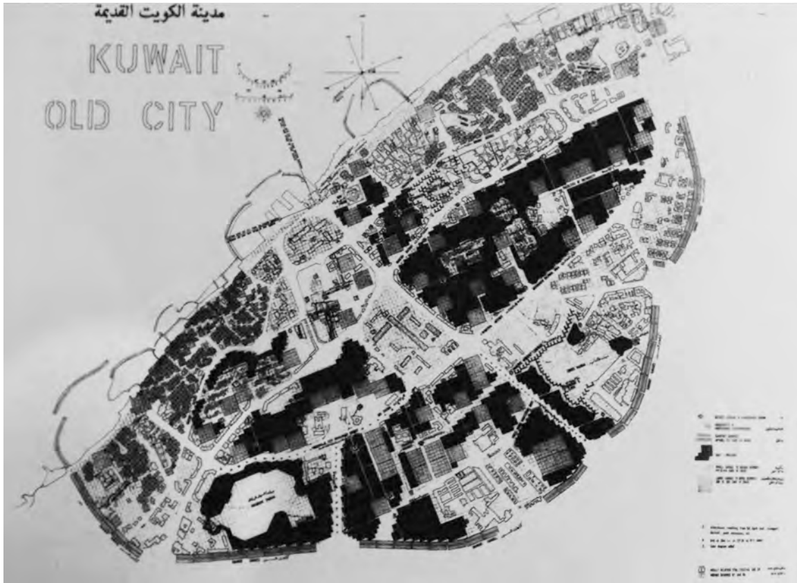
Figure 120: A detailed plan of Alison and Peter Smithson's mat-building of Kuwait (the voids are represented in white/ lighter shade). Source: Alison and Peter Smithson's Archive, Frances Loeb Library at Harvard Graduate School of Design, Cambridge.
