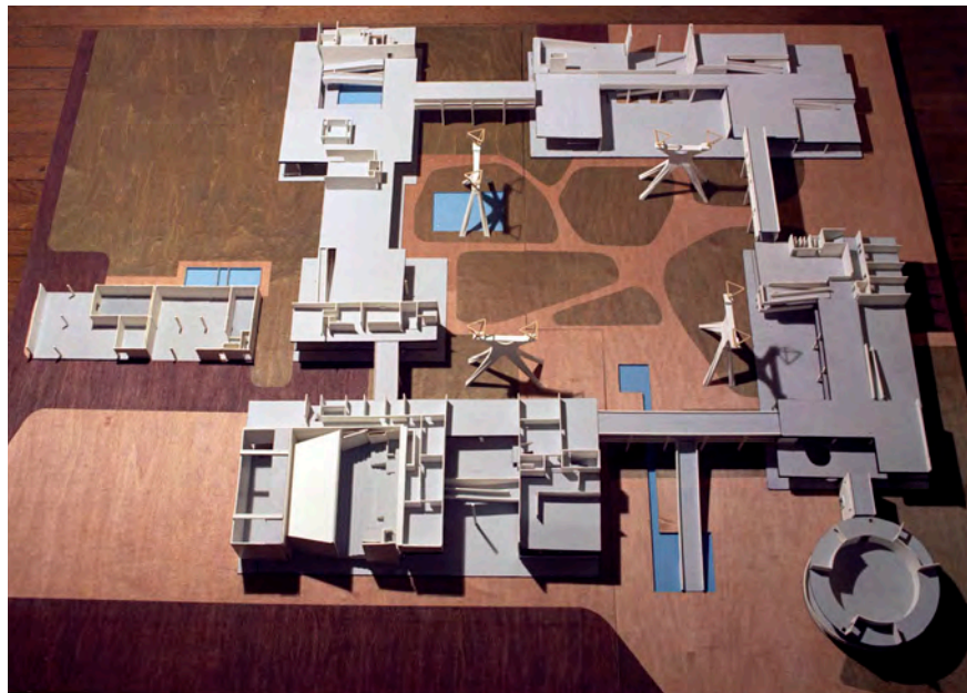
Figure 125: Model photograph of Michel Écochard’s Kuwait National Museums, the image shows the bridges (streets in the sky) connecting various buildings of the museum’s complex. Source: Aga Khan Award for Architecture.
