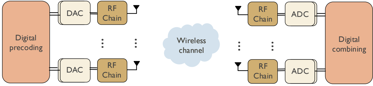
Figure 1.1. Block diagram of a conventional multiple-input-multiple-output (MIMO) architecture, where each antenna at both receiver and transmitter is connected to a radio frequency (RF) chain and data converters. The precoding and combining operations are performed entirely in the digital domain. While scaling up the array aperture, the fully digital architecture leads to a high power consumption as the number of power-hungry components in the RF chain increase commensurately with the number of antennas.
