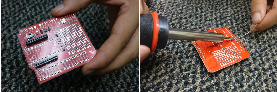
Figure 16. Soldering the headers into the XBee shield for Arduino .
