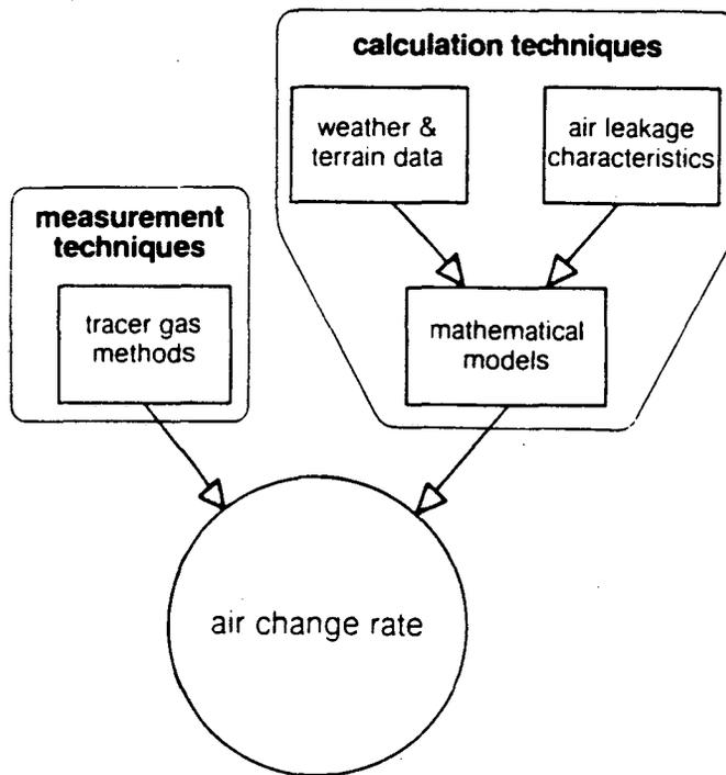
**Fig. 2: Alternative Ways of Determining Infiltration [1]**
