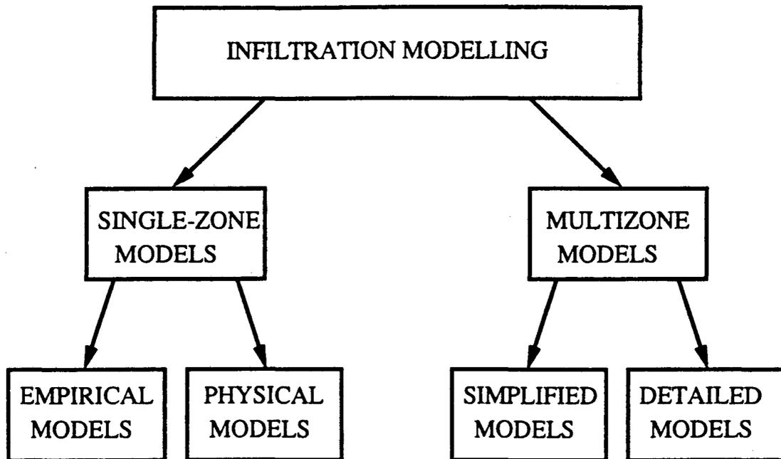
**Fig. 3: Categorizing Infiltration Models**
