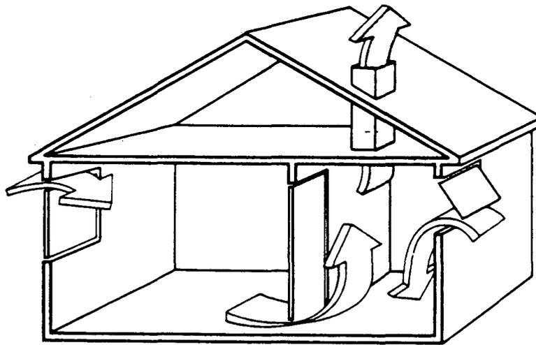
**Fig. 6:** *Example of a simple Multizone Structure [1]*
