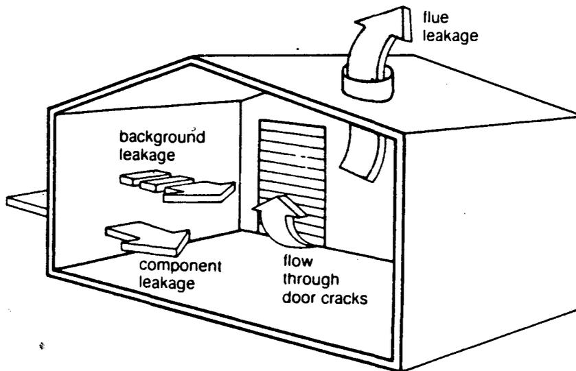
**Fig. 4: Example of a Single-Zone Building [1]**
