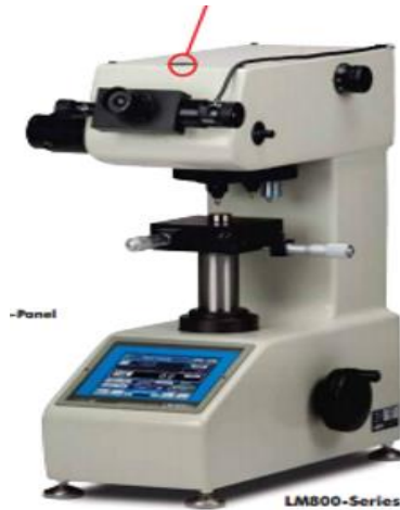
Figure 4.2 Hardness tester LM 810-AT model manufactured by LECO Corporation 135 .
