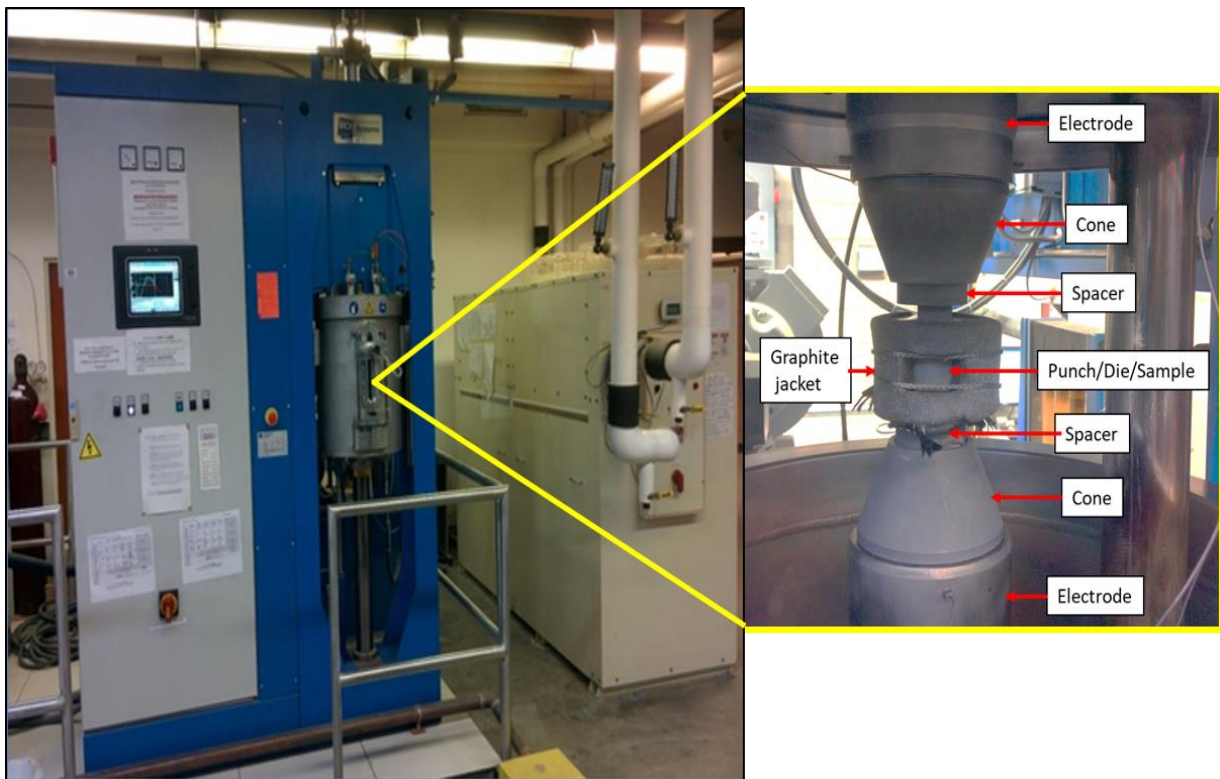
Figure 3.4 Photograph of spark plasma sintering furnace at Alfred University, New York. The graphite die-cone arrangement along with the sample inside the die is shown in the inset picture to the right.
