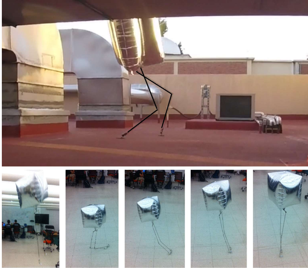
Fig. 6.3: The robot landing with legs highlighted for clarity (Top). Passive model falling and recovering (Bottom-Sequence left to right).
