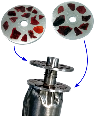
FIG. 7. KYbSe 2 sample used to measure the low-energy spin excitations on CNCS. 20 crystals were coaligned and glued to two aluminum plates (top) which were then screwed to a copper rod (bottom). The different crystals are different shades of red because of their different thicknesses.
