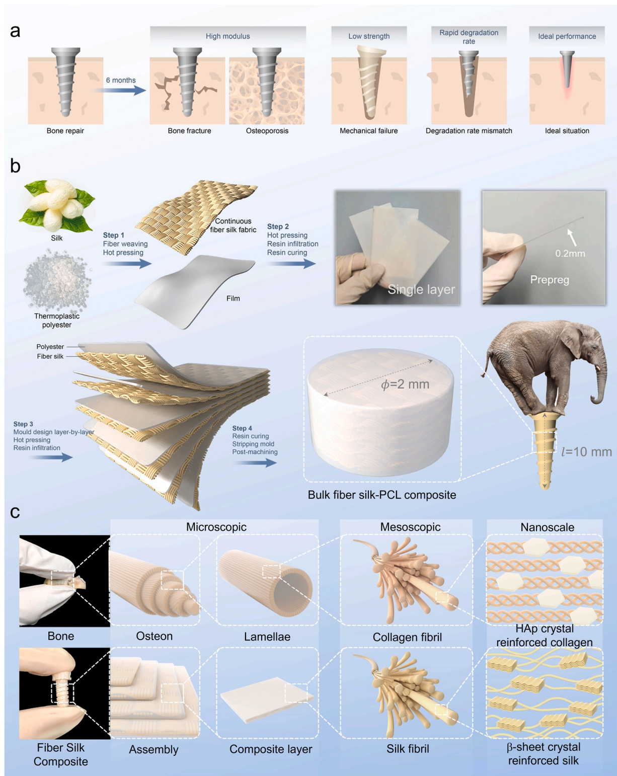
Fig. 1. Illustration of the preparation process of the CFSCs. (a), Different bone repair and regeneration effects induced by incompatible properties of bone graft materials. (b), Utilizing a physical processing approach or thermal and pressure molding, natural continuous fiber silks are prepared into three-dimensional silk-based materials that retain macroscopic continuity and the multi-level structure of continuous fiber silk. Step 1: Preparation of silk fabric and the thermoplastic polyester film. Step 2: Hot-pressing or pressure-driven melt fusion to produce single layer prepreps. Step 3: Prepreps are assembled layer-by-layer, and bulk CFSCs are prepared by a 2nd hot-pressing. Step 4: Post-machining to achieve desired shapes. (c), Illustrations of the multi-scale hierarchical structure of CFSC and natural bone. In CFSC, continuous fiber silk in the composite lamella is further composed of micro-/nanofibers with a semicrystalline morphology; in bone, the bone lamella is composed of collagen fibrils with tropocollagen nanorods and hydroxyapatite nanocrystals. Such unique hierarchical structure forms the basis for their surprising performance.
