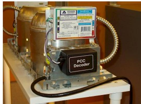
Figure 4. Closeup of the PCC Decoder and the electronic dimming ballast (0-10 VDC) controlled by the system.
