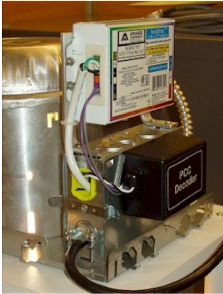
Figure 5. Closeup shot of the PCC Decoder showing the electrical connections between the decoder and the ballast.
