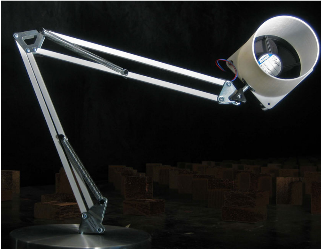
Figure 2.9: Fan version 2.4 "Fankenstein" is the result of combining the best-performing inlet and outlet combinations and mounting them on a swing-arm base.
