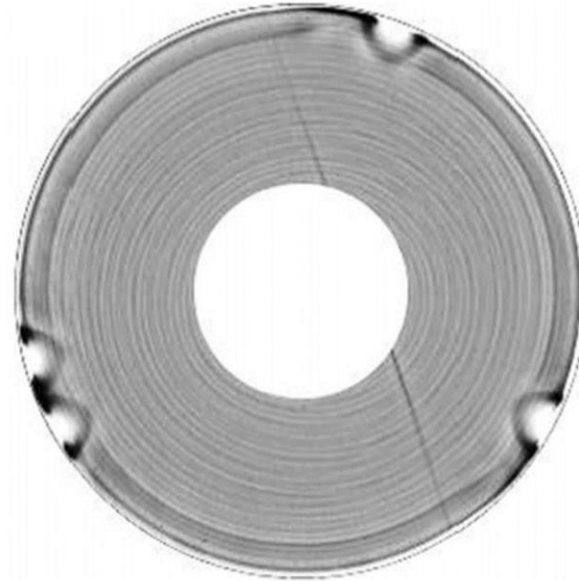
Figure 2.10 Optical surface analysis image of a disk surface with different lubricant thickness measured. Q-polarized light is used [128]
