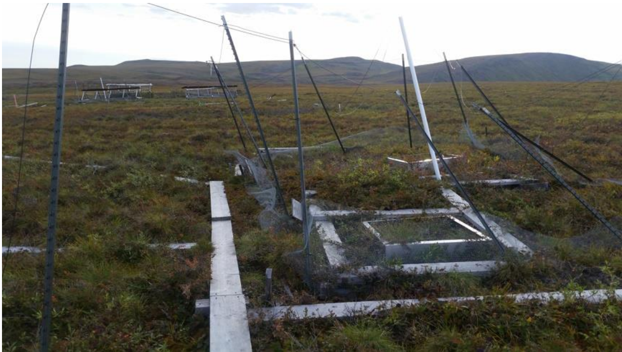
Figure 40 Even t-posts bend and collapse over repeated Arctic winters.
