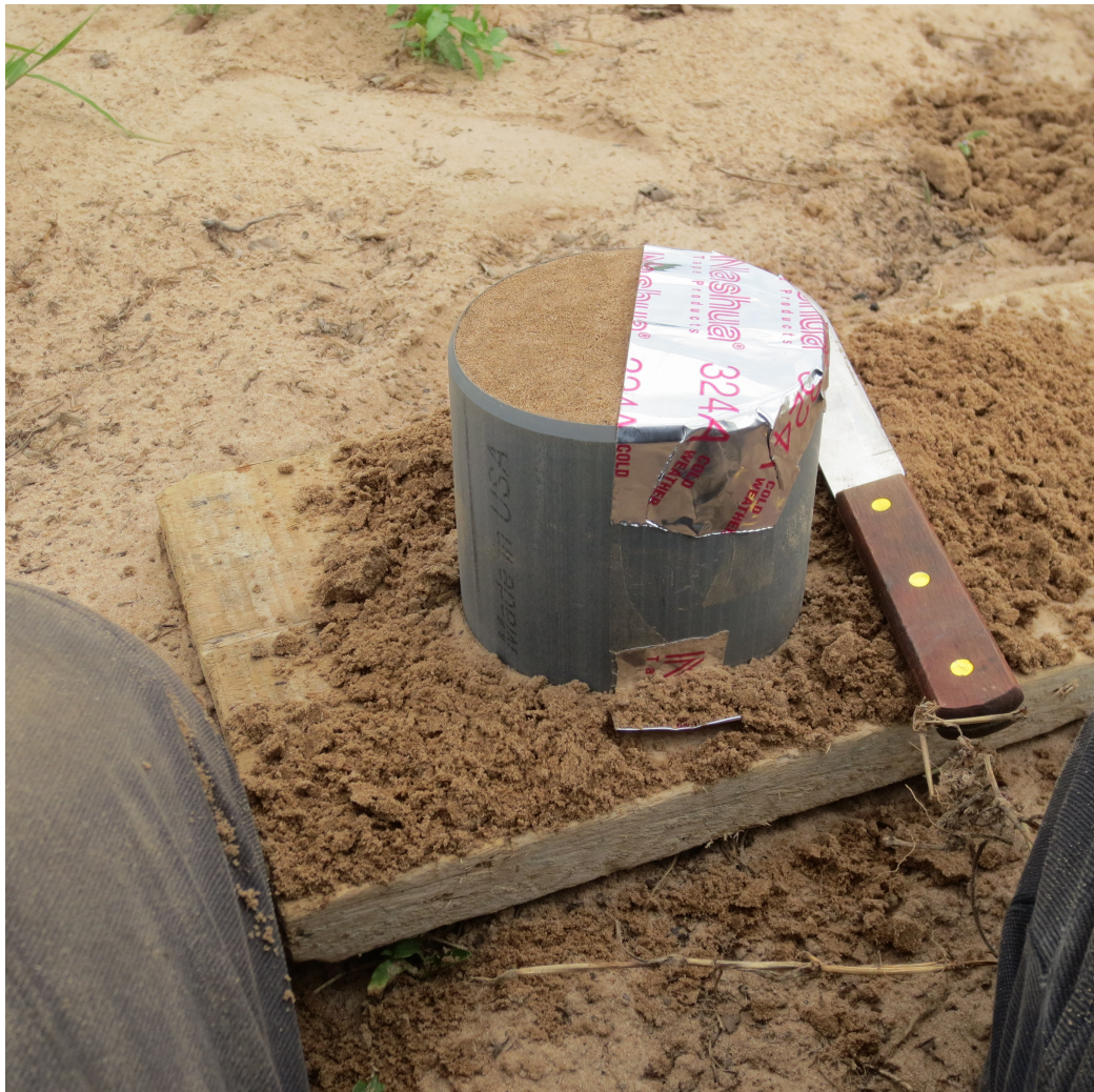
FIGURE B.2. Preparing the microlysimeter in the field. Heat conductive, waterproof tape being applied to the bottom side of lysimeter after trimming soil. Outer diameter of lysimeter is 10.7 cm
