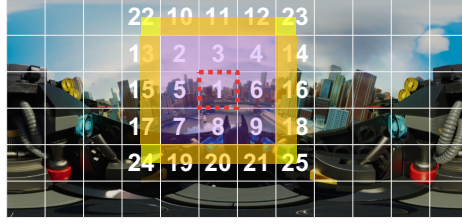
Figure 3.10: Illustration for the calculation of FOV probability p_{fov} from viewpoint probability p_v .
