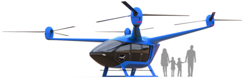
Fig. 14: Conceptual design of an electric quadrotor (Ref. 20).
