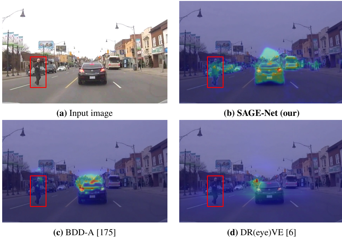
Figure 3.1. Predicted saliency map for different models (Best viewed in color). The bounding box shows a pedestrian illegally crossing the road and is prone to accidents. While other models only capture the car ahead (partially), the proposed model can completely learn to detect both the car and the crossing pedestrian.
