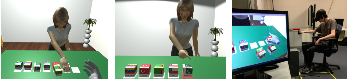
Figure 4.5: We present an autonomous virtual trainer that can assist users to learn a given task by using different feedback strategies involving manipulation (left) and pointing (center). Immersed users interact with the virtual trainer with voice commands while manipulating virtual cubes using Rift controllers in order to learn the task (right).
