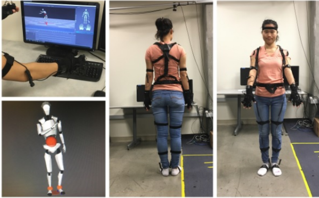
Figure 3.3: Perception Neuron full-body motion capture suit setup.
