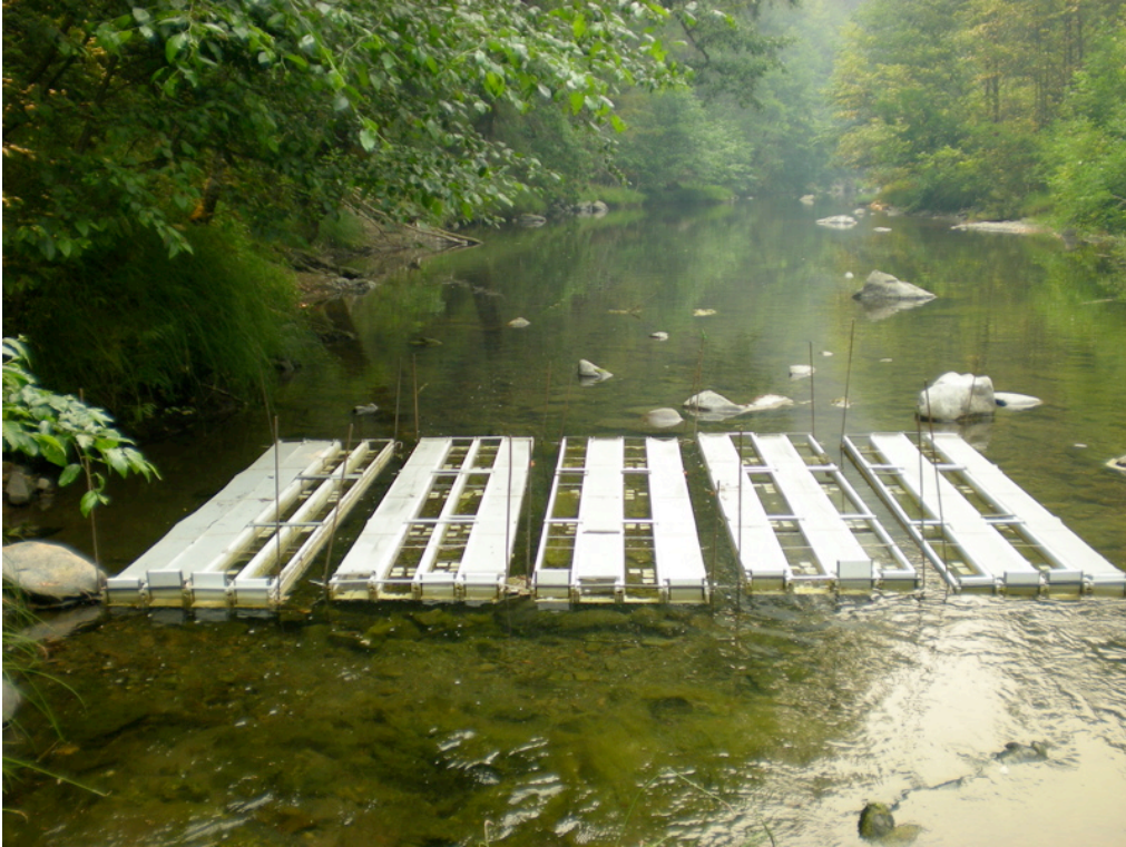
Figure 1. Stream Channel Experiment. View looking downstream, showing 20 channels in the South Fork Eel River. Each channel is 3 m long x 15 cm wide x 15 cm deep. The velocity gates are visible at the head of each channel, with those in the raised position on the Faster treatment channels and those in the lowered position for the Slow treatment channels. Shade cloth covers the Dark treatment channels. Cobbles and tiles are visible in the Light/unshaded channels. Five channels were randomly assigned to each treatment (channels are numbered from the left): Slow, Dark —channels 1, 8, 12, 13 and 20; Faster, Dark —channels 2, 5, 10, 15 and 18; Slow, Light —channels 4, 7, 9, 16 and 17; Faster, Light —channels 3, 6, 11, 14 and 19.
