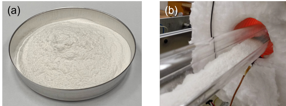
Figure 5.1: (a) Microcrystalline cellulose powder tested in this work and (b) cellulose powder shown in the quartz boat inserted in the quartz tube during an experiment.
