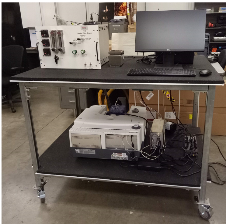
Figure 2.5: Image of Thermo Scientific Nicolet iG50 Fourier-transform infrared (FTIR) spectroscope placed on a cart.
