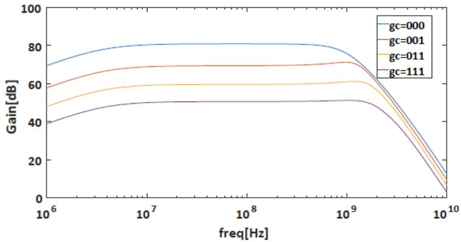
Figure 2.5: Frequency response of the TIA for four gain settings.
