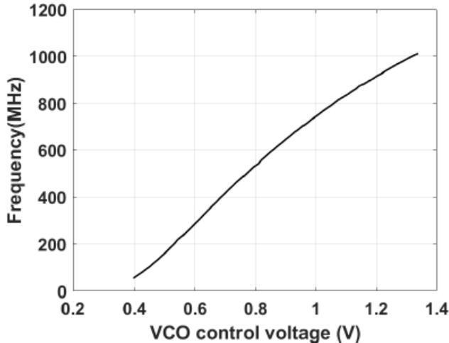
Figure 2.3: Frequency vs. control voltage curve.
