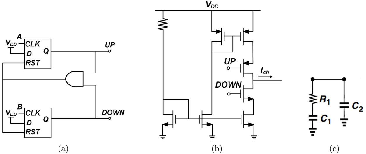
Figure 3.4: (a) Block diagram of the PFD; (b) charge-pump circuit; (c) loop filter.
