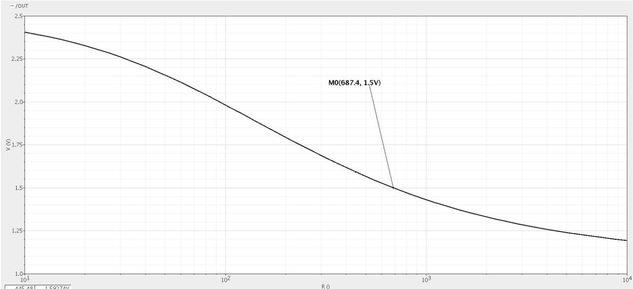
Figure 4.13: Output node's dc value vs. the resistor value at the source.
