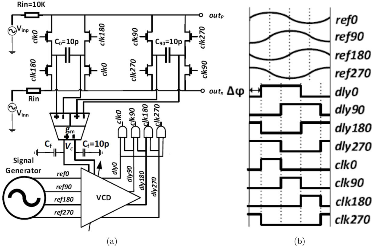
Figure 2.7: (a) Block diagram of the phase detector; (b) clock and pulse signals.
