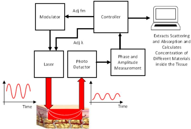
Figure 1.2: fd-NIRS system block diagram.
