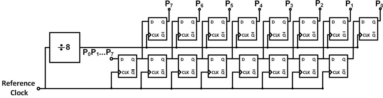
Figure 4.9: 8-bit serial-to-parallel converter's schematic.
