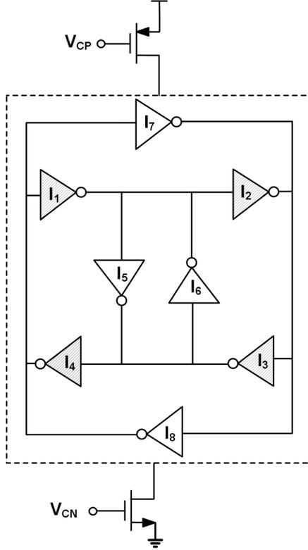
Figure 2.2: QRVCO's schematic.
