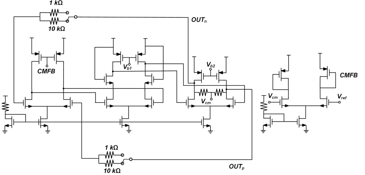
Figure 3.5: Schematic of the TIA.
