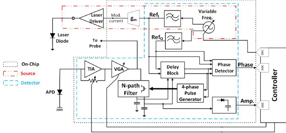
Figure 2.1: 1<sup>st</sup> version chip's block diagram.
