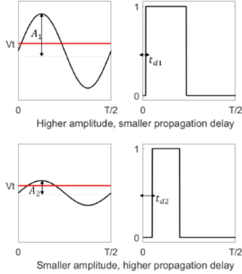
Figure 3.2: Amplitude dependent time-offset of limiting amplifier.
