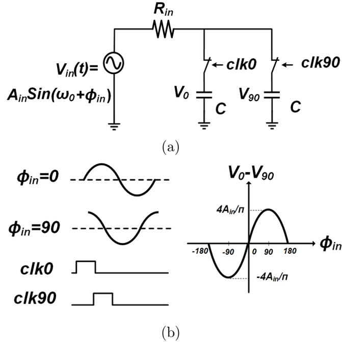
Figure 2.8: (a) Simplified behavioural model of 4-path filter; (b) two different input phases with  $(V_{C0} - V_{C90})$  vs.  $\phi_{in}$  characteristics.
