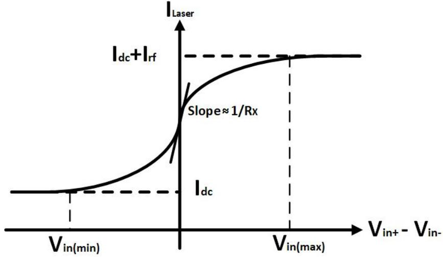
Figure 4.19: I-V Characteristics.
