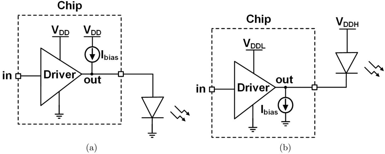
Figure 4.16: (a) Common-cathode driving topology; (b) common-anode driving topology.
