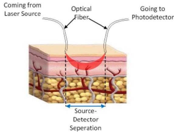
Figure 1.1: DOI system configuration.
