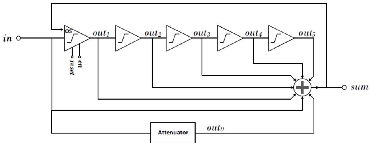
Figure 2.9: Block diagram of the amplitude detector.
