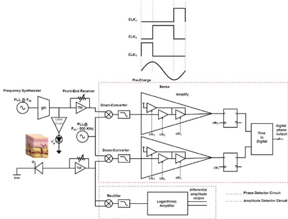
Figure 3.1: 2<sup>nd</sup> version chip's block diagram.
