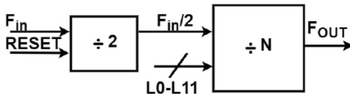
Figure 3.3: Frequency divider building block.
