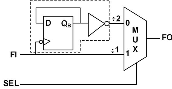
Figure 4.6: Concept of a (2/1) divider cell.
