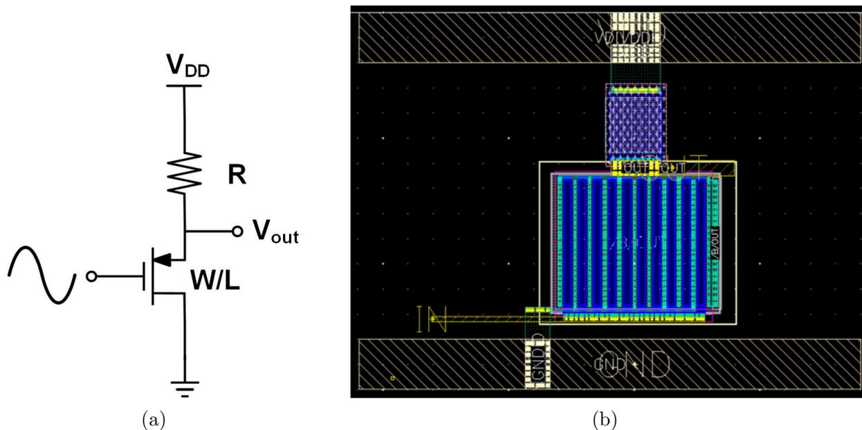
Figure 4.12: (a) Schematic of the source follower; (b) layout of the source follower.
