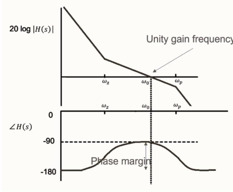
Figure 4.10: Bode plot of the open loop transfer function of the PLL.
