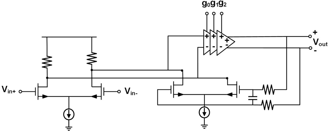
Figure 2.6: Schematic of the VGA.
