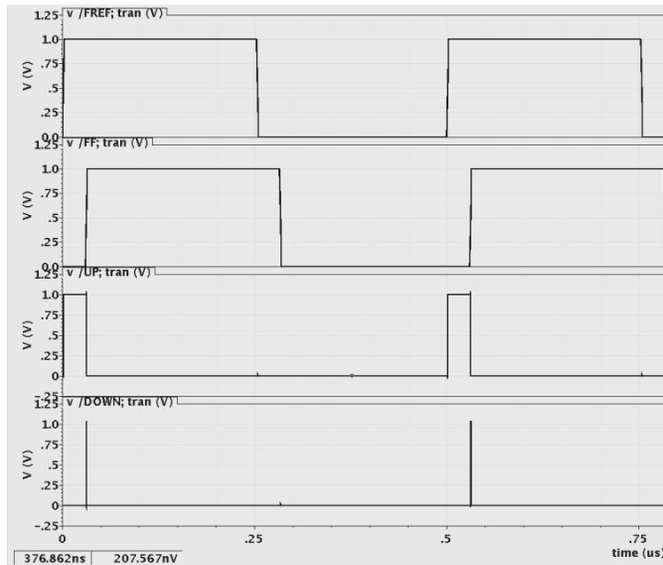
Figure 4.4: Transient response of the PFD.
