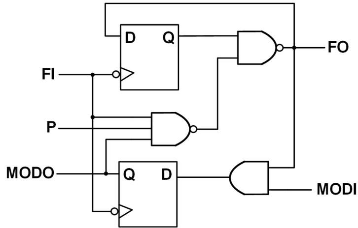
Figure 4.7: Proposed (2/1) divider's block diagram.
