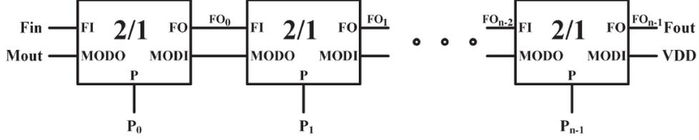
Figure 4.5: Proposed N-stages programmable frequency divider
