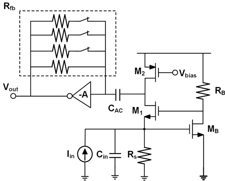
Figure 2.4: Schematic of the TIA.
