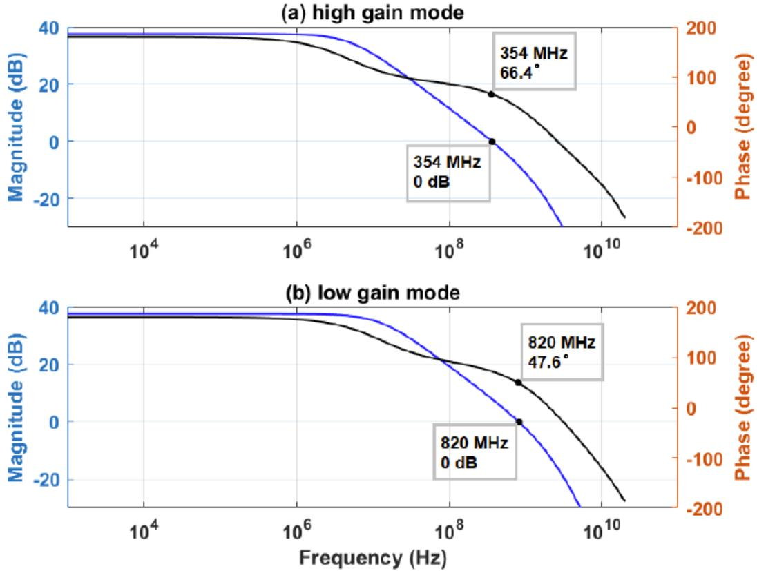
Figure 3.6: Bode plot of the open-loop TIA.
