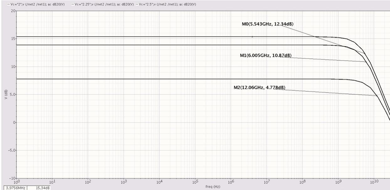
Figure 4.15: Ac response of the VGA for  $V_C = 2.5V$ ,  $V_C = 2.25V$ , and  $V_C = 2V$ .
