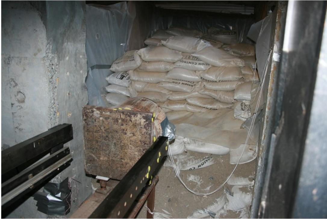
Figure 4.2: Specimen Catcher Pit
