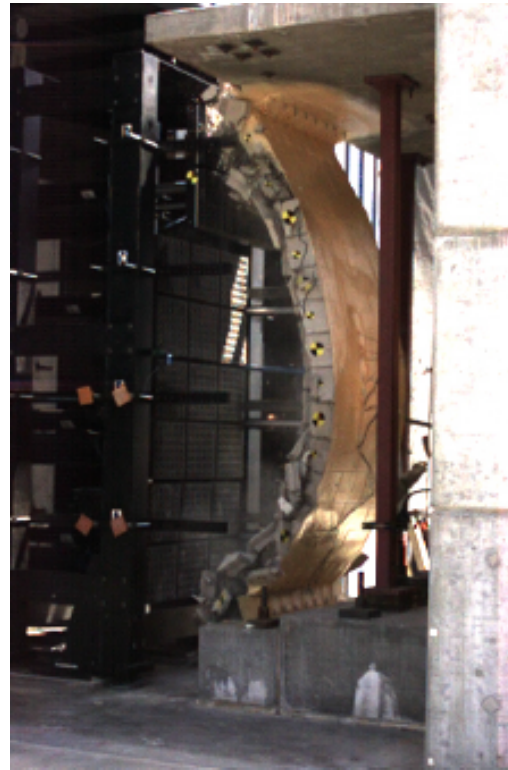
Figure 3.7: CMU Wall Test with the Blast Simulator (taken directly from [14])
