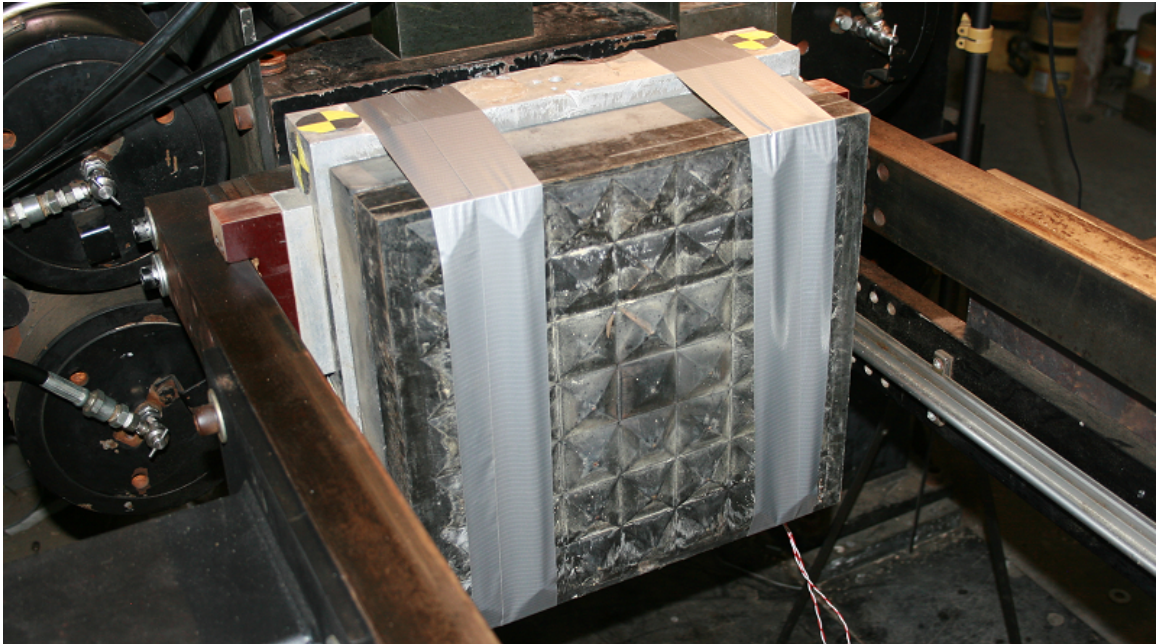
Figure 4.20: Double Programmer Impactor Configuration
