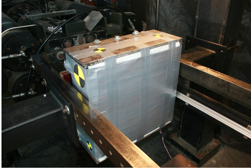
Figure 4.48: Impacting Mass Assembly with Confined Sand
