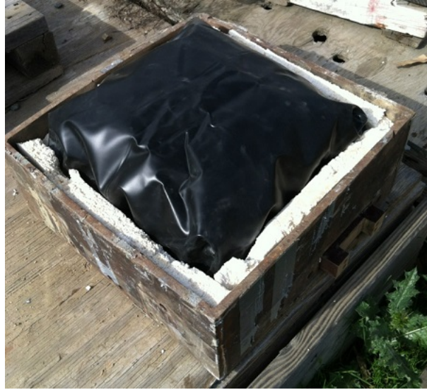
Figure 4.47: Confining Box with Sand Bladder
