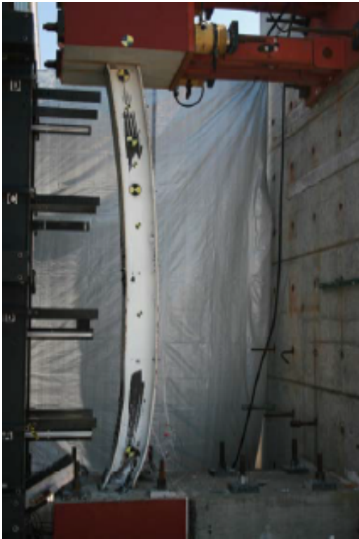
Figure 3.6: Steel Column Test with the Blast Simulator (taken directly from [18])
