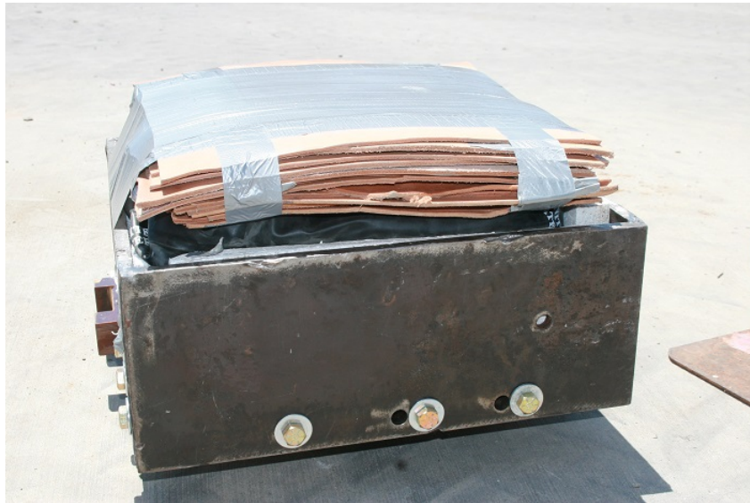
Figure 4.57: Leather and Sand Combination as Impact Medium
