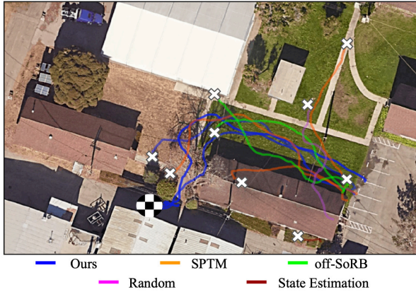
Fig. 2: Qualitative Results in the urban Environment: Each approach was directed to a visual goal \sim 50\text{m} away (marked by checkerboard circle) – with 3 runs per approach. ViNG is the only approach that is consistently able to reach the goal while avoiding collisions or getting stuck.
